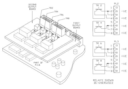
View illustrating mounting positions of dual opto-isolated boards Opto-isolated output PCB connectors
